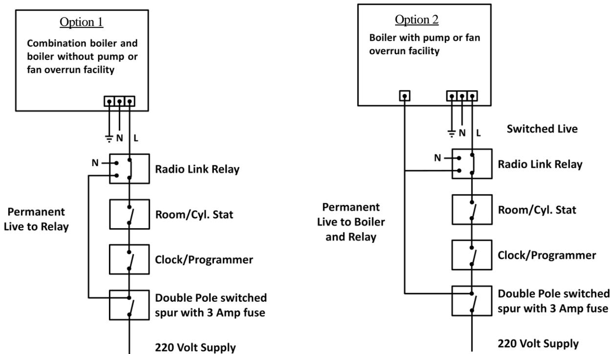
The wireless receiver relay device must be connected via a spur/switch which needs to be doubled poled and fused at 3 amps. It is recommended that the wireless receiver relay or type A detector be the last control device in the wiring circuit before connection to boiler.
